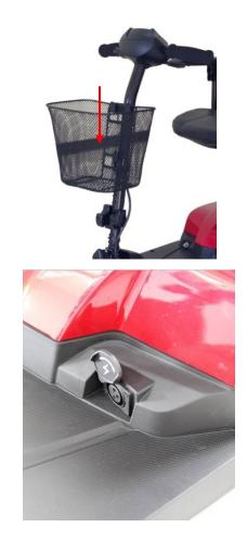
Your transport scooter can be disassembled into five sections without tools: the seat, basket, battery pack, front section and rear section. Please be sure to follow these steps to properly assemble and disassemble your scooter.
