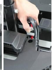
Step 4: Place the red cover back onto the base of the scooter.
